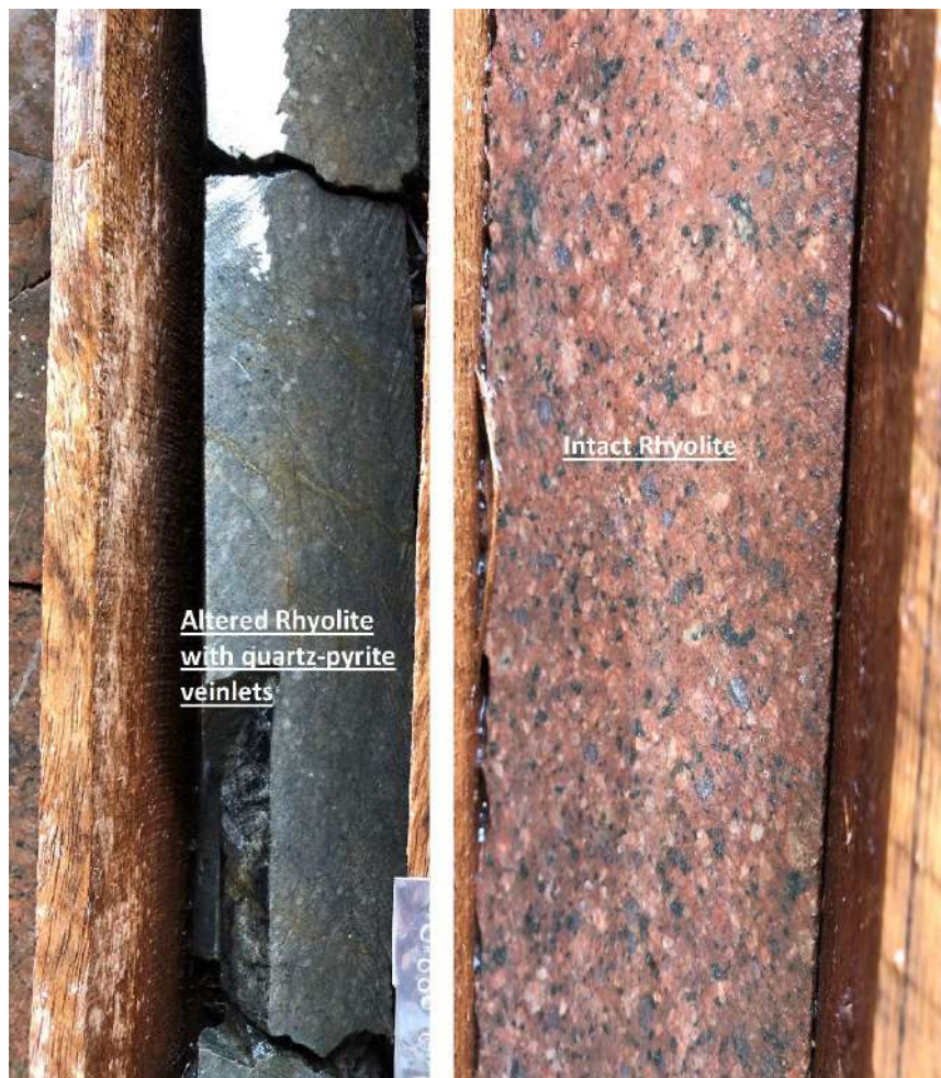
Figure 8-1 Altered and Intact Rhyolite in Core Boxes, Cajueiro
