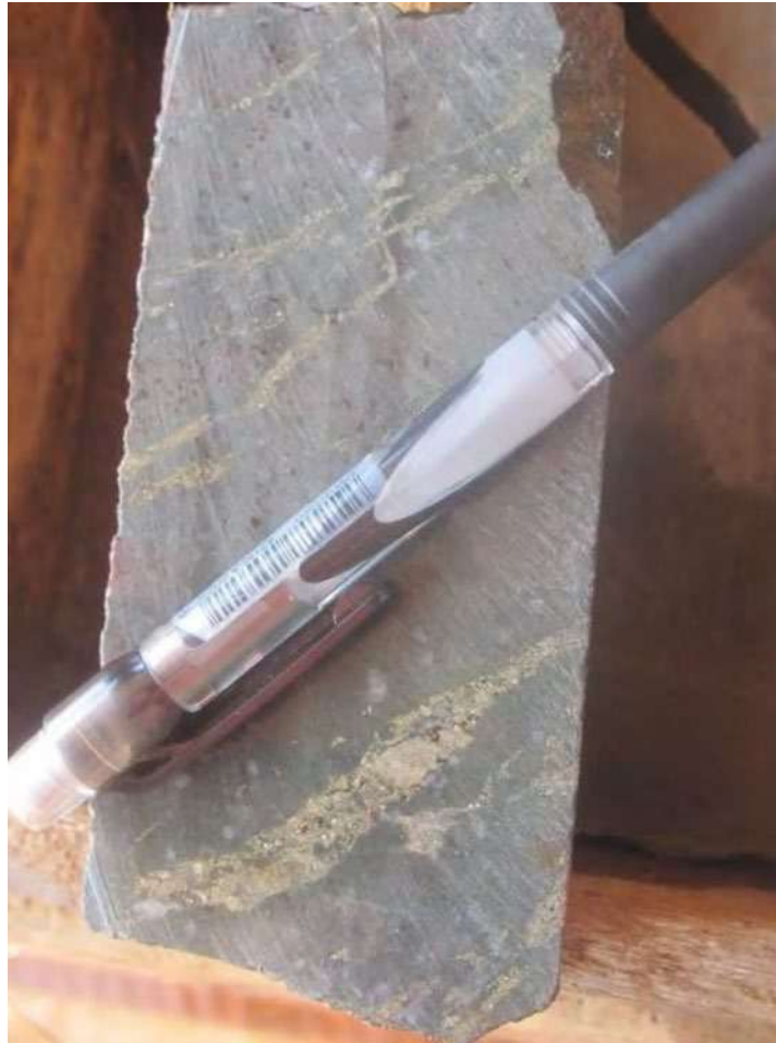
Figure 8-2 Pyrite Stringers in Altered Rhyolite in Cut Core Sample, Cajueiro
