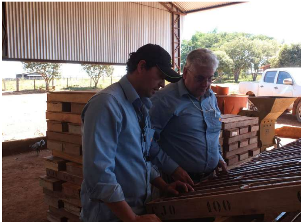
Figure 10-1 Example of Core Logging at Site
